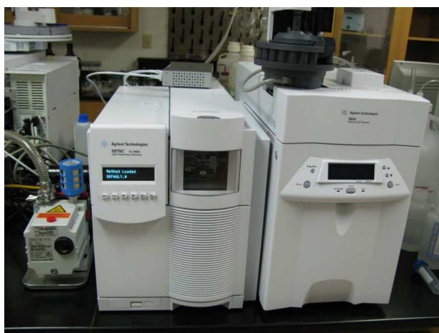
Figure 13: Gas chromatography (GC)
