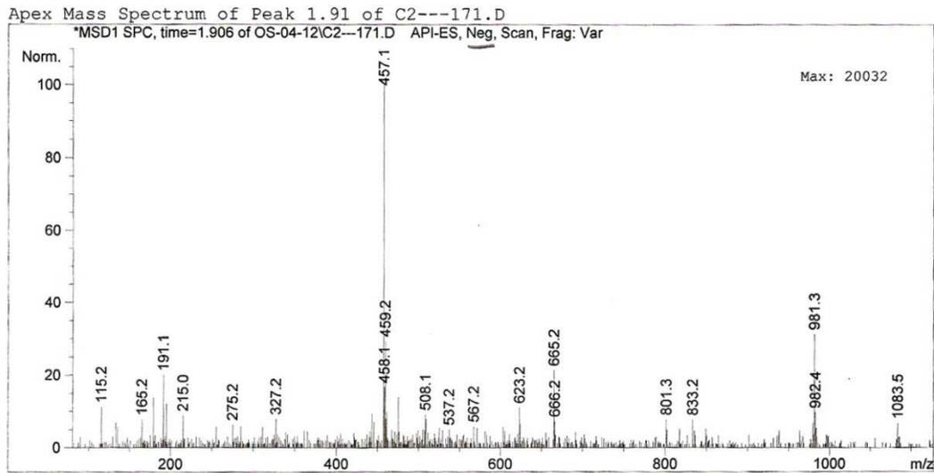
**Fig: 3(b)** Mass spectra obtained in negative ion mode fragmentation of Phenolic extract of *Svensonia hyderbadensis* (Sample-2)
