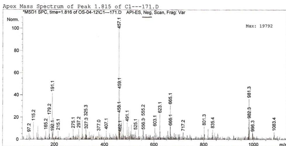
**Fig: 2(b)** Mass spectra obtained in negative ion mode fragmentation of Phenolic extract of *Svensonia hyperbadensis* (Sample-1)
